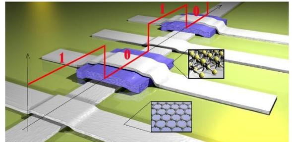
*Schematic of a printed logic memory device made from ink-jet graphene*
