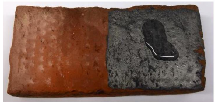
A brick half with and half without a reduced graphene oxide coating, showing the ability of water to permeate into the non-coated brick.
